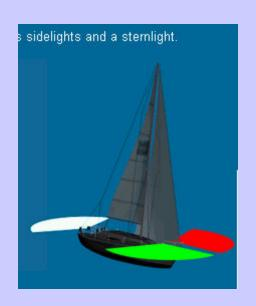
A <u>sailing vessel < 20m. long</u> may show combined sidelights & sternlight (tricolour) at the masthead. <u>The tricolour must not be shown with any other lights.</u>
